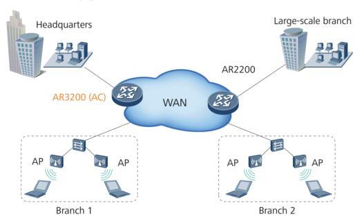
The AR3200 routers integrate AC (Access Controller) functionality, which can manage the wireless AP (Access Point) in wireless LAN. AR2200 supports rich certification and flexible user access control, which can provide security access guarantee for Wi-Fi users. The rich wireless capabilities integrated in one device, this can realize centralized management of wired and wireless networks, to meet the requirements of different scale enterprises networks.
