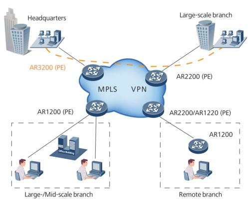
The AR3200 routers are well suited to serve as PEs in the headquarters office of a large enterprise. The MPLS L3 VPN segregates services by type. The AR3200 routers feature flexible deployment, fast distribution, and secure transmission of VPN services, as well as supporting enterprise service operation over networks.
